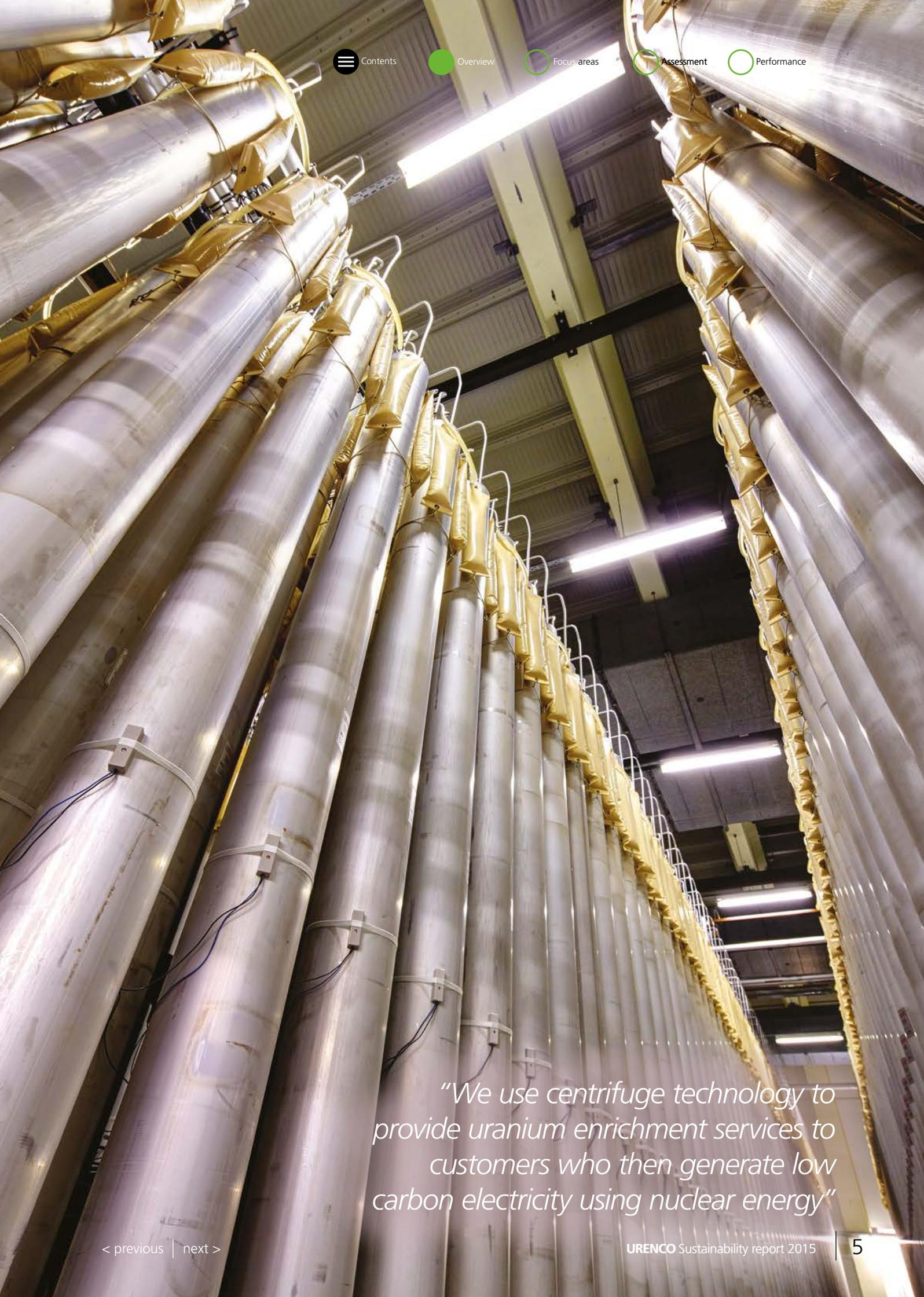
*“We use centrifuge technology to provide uranium enrichment services to customers who then generate low carbon electricity using nuclear energy”*
